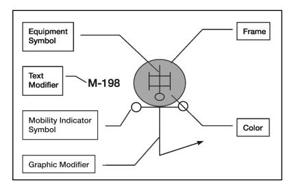
Figure 6-1. Equipment Symbol Components
