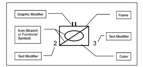
Figure 5-1. Unit Symbol Components
