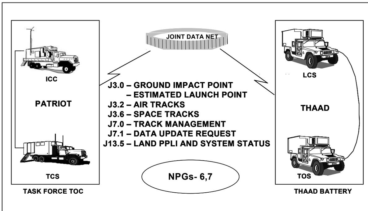
**Figure C-12. Joint Data Net**
