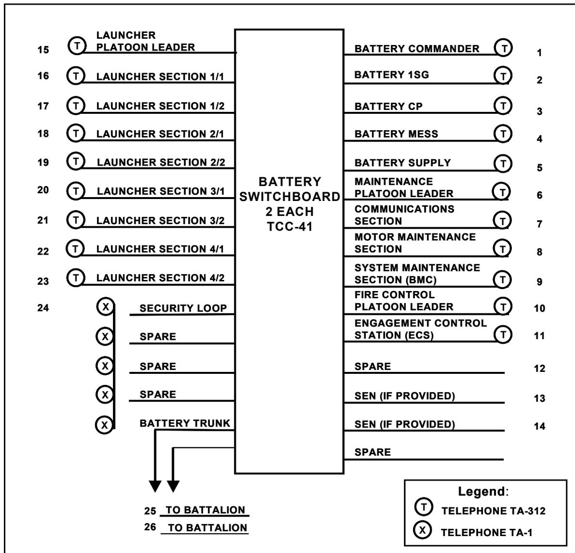
Figure C-9. Battery Switchboard Connections
