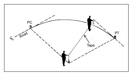
Figure I-3. Find the Radius with a Tape Measure
