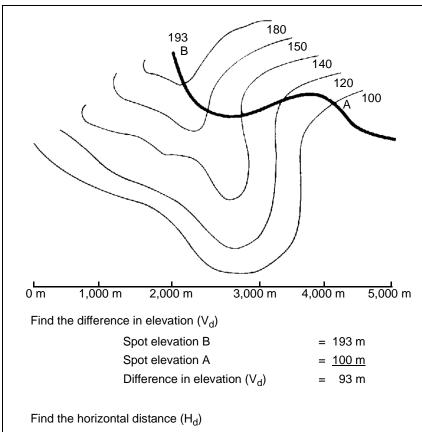
Road distance A to B (use a piece of paper and a graphic scale as shown in FM 21-26) = 3,720 m
