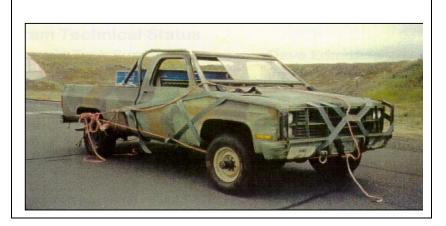
Figure L-14. Vehicle Entrapped in a PVAB
