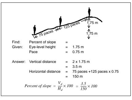
Figure I-7. Determine the Slope Using the Pace Method
