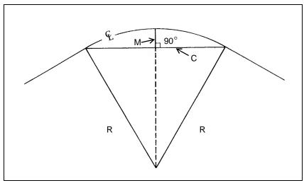
Figure I-4. Determine a Curve Radius
