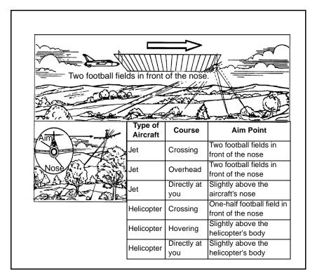
Figure 3-3. Rules for Selecting the Aim Point
