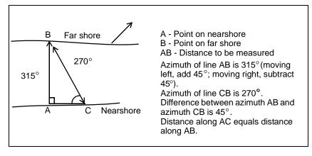
Figure I-8. Determine Stream Width
