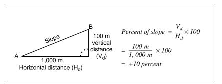
Figure I-5. Calculate the Percent of Slope
