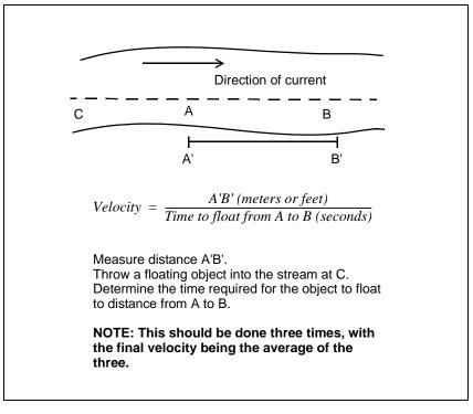
Figure I-9. Determine Stream Velocity
