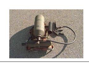
Figure L-10. M33A1 Riot Control Disperser Filled With CS or CR
