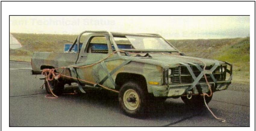
**Figure L-14. Vehicle Entrapped in a PVAB**
