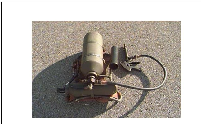
**Figure L-10. M33A1 Riot Control Dispenser Filled With CS or CR**
