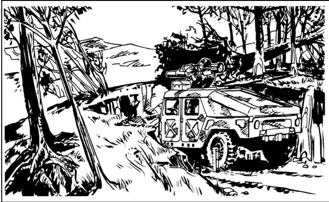
Figure D-6. Excavated hull-down position
