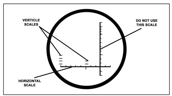
Figure 8-6. Mil scale on M17 binoculars.
