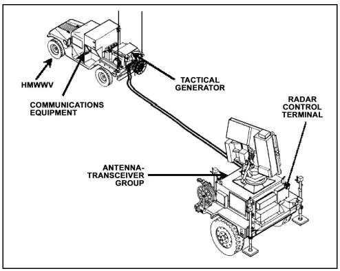
Figure 8-22 Sentinel radar system.
