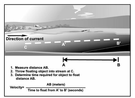
Figure A-5. Measuring stream velocity.
