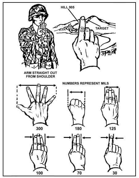
Figure 8-7. Hand and fingers used to determine deviation.
