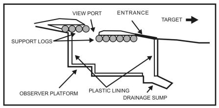
Figure 5-31. Bunker-type underground observation post.
