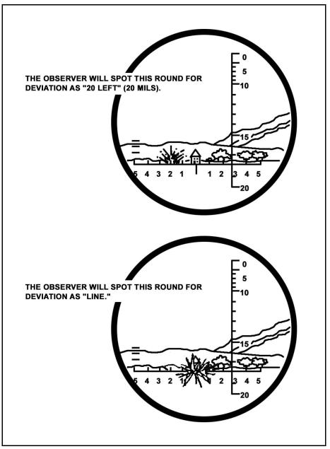
Figure 8-8. Deviation spotting with binoculars.
