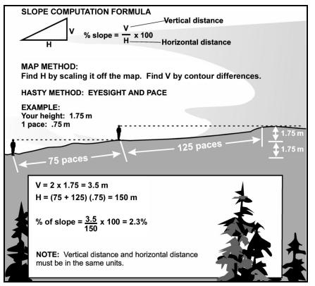
Figure A-6. Slope computation (road gradient).
