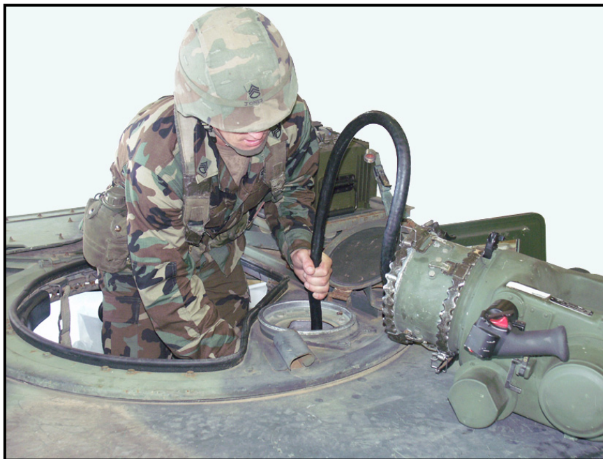
Figure 3-3. Coil cable passes through pedestal mount.
