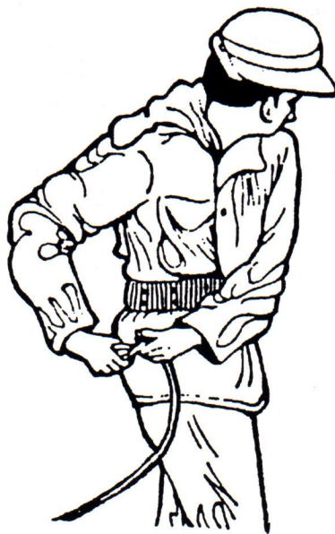
Holding the fuse while crimping.
