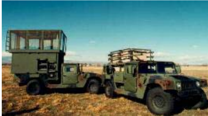
Figure E-1 AN/MSN-7 Tower Restoral Vehicle
