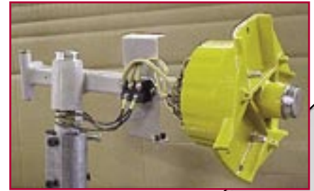
Rotor, stator, diode rectifier, slip rings, and bearings exposed on a Bergey XL.1 1 KW generator.
