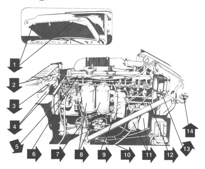
This Systematic Inspection Procedure is designed to make it easier for you to inspect and check your 2½ ton truck to help keep it "always ready" to move. Simply follow the direction of the arrows as you make your inspection.
