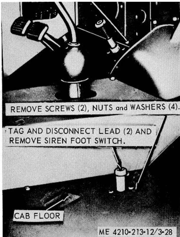
Figure 3-28. Siren foot switch, removal and installation.
