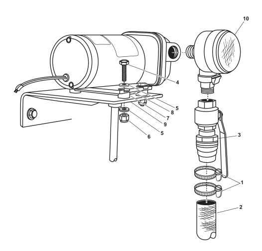
Figure 2. Fresh Water Flush Pump (Inlet Side)
