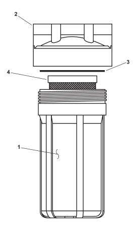
Figure 1. Charcoal Filter Assembly
