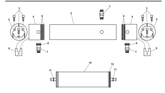
Figure 3. RO Membrane and Vessel Subassembly Repair
