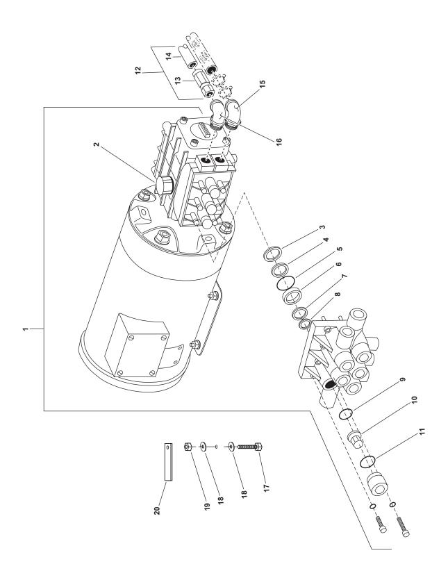
Figure 5. High Pressure Pump
