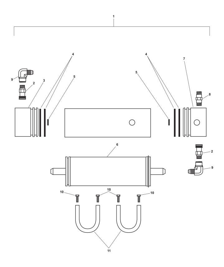
Figure 6. Membrane and Vessel Assembly
