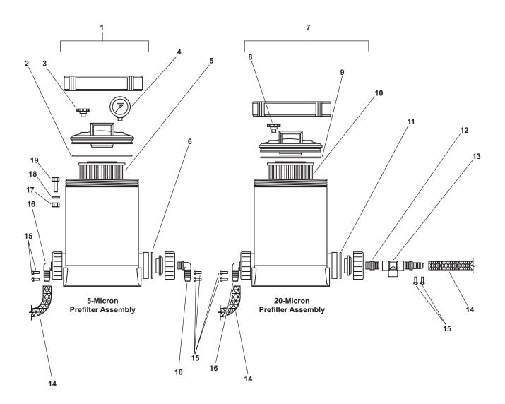
Figure 4. Prefilter Assembly
