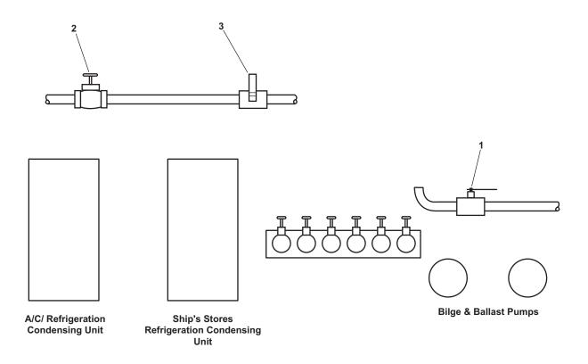
Figure 10. Potable Water Valves on AMS 2 Aft Bulkhead
