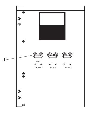
Figure 7. 24 Vdc Control Panel
