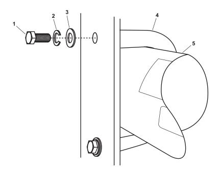
Figure 2. Membrane Mounting Hardware
