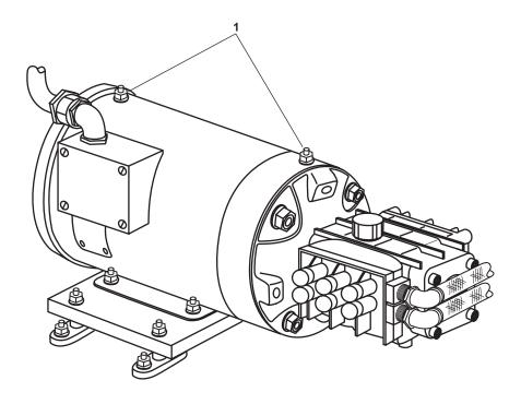
Figure 5. High Pressure Pump Grease Fittings
