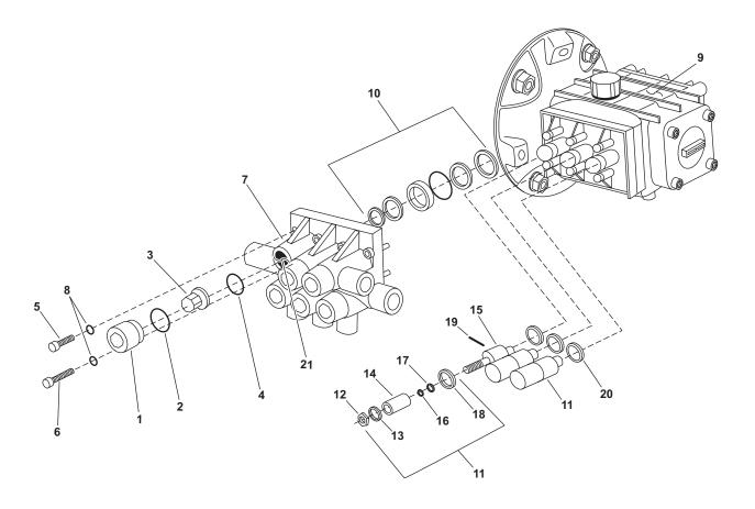
Figure 1. High Pressure Pump
