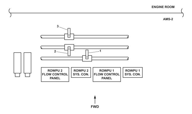
Figure 11. ROWPU System Valves as Viewed from Above
