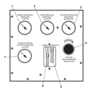
Figure 3. Flow Control Panel Controls and Indicators
