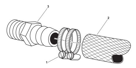
Figure 1. Low Pressure Fitting, Hose, and Clamp
