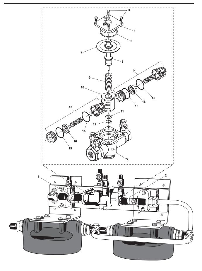
Figure 8. Backflow Preventer Valve
