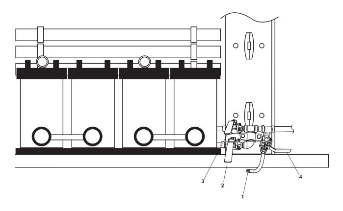
Figure 9. ROWPU Filter Inlet Valves
