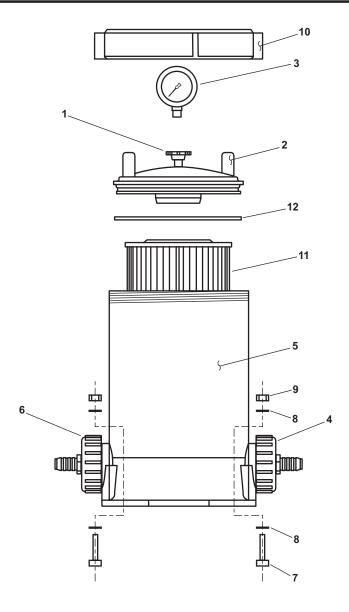
Figure 1. Filter Assembly
