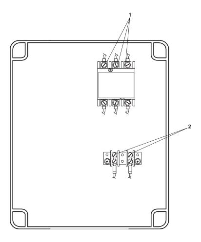
Figure 2. System Controller Terminal Boards
