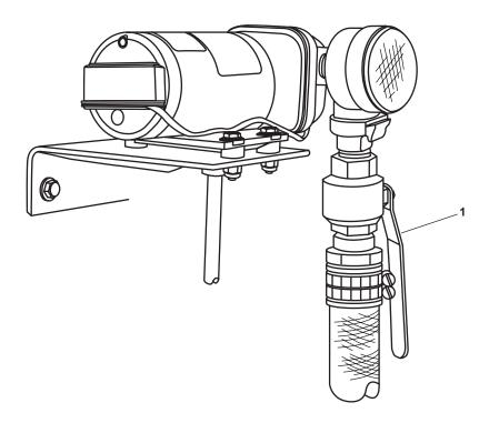
Figure 14. Fresh Water Flush Pump Outlet Valve
