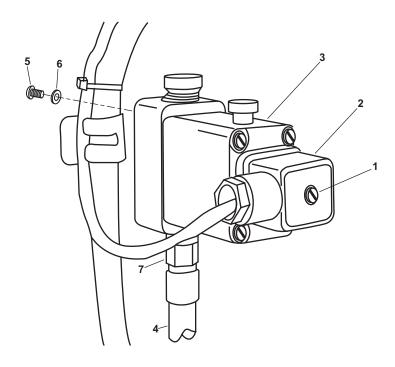
Figure 7. Fresh Water Flush Diverter Valve
