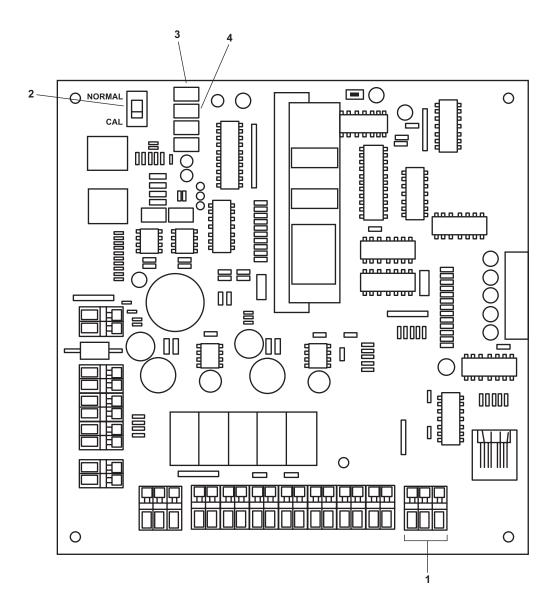
Figure 3. System Controller Motherboard and Connections
