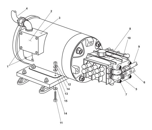
Figure 1. High Pressure Pump
