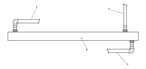
Figure 1. Reverse Osmosis Membrane and Vessel Subassembly
