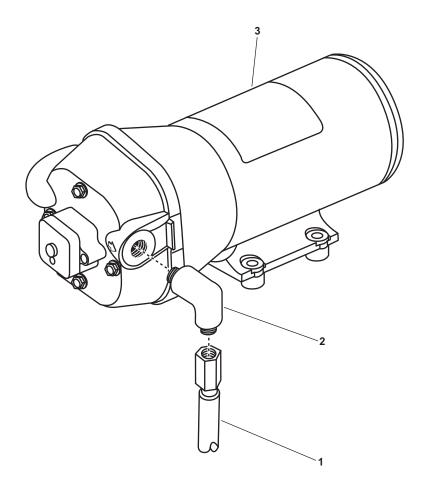
Figure 3. Fresh Water Flush Pump (Outlet Side)
