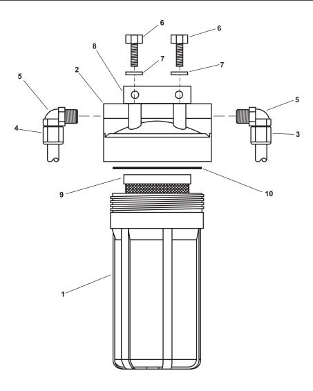
Figure 1. Charcoal Filter Assembly
