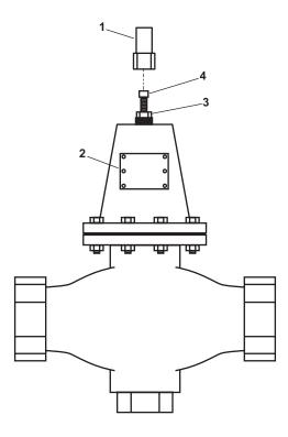
Figure 2. ROWPU System Pressure Regulator Valve
