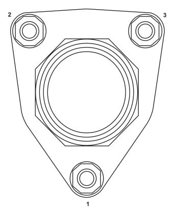
Figure 2. Torque Pattern for Sil Braze Ball Valve
