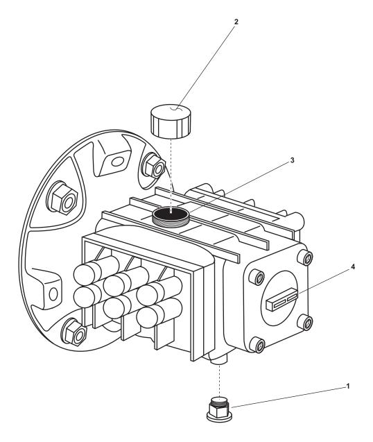
Figure 1. High Pressure Pump
