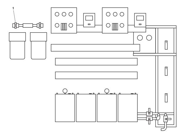
Figure 2. ROWPU System Front View
