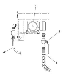
Figure 2. Fresh Water Flush Pump
