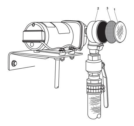
Figure 4. Fresh Water Flush Pump Inlet Strainer
