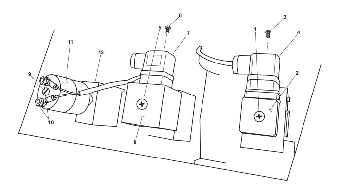
Figure 6. Flow Control Panel, Top View
