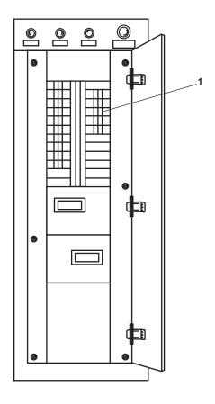
Figure 2. Load Center Distribution Panel
