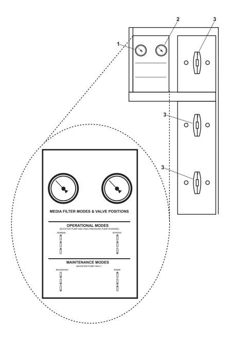
Figure 5. Media Filter Gauges and Maintenance Valves
