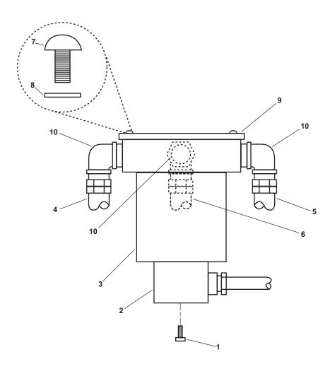
Figure 8. Product Water Diverter Valve
