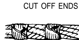
6 BEND TWISTED PORTION DOWN AGAINST ROPE
