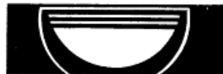
Figure 3.1 Sight reticle, M103A1 sight.
