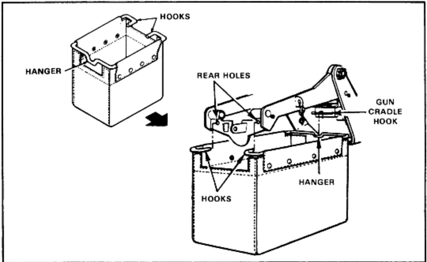
Figure 3-26. Attachment of empty case catch bag.
