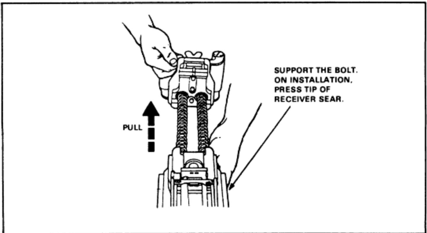
Figure 2-11. Removal of bolt and backplate assembly.
