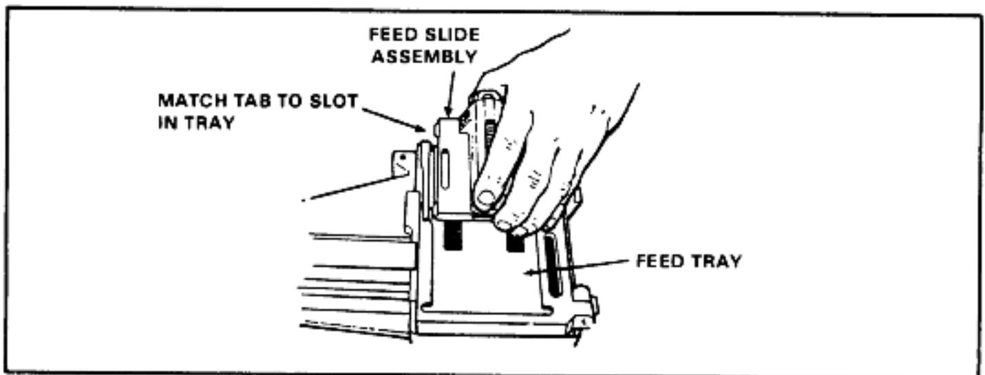
Figure 2-8. Feed slide assembly.
