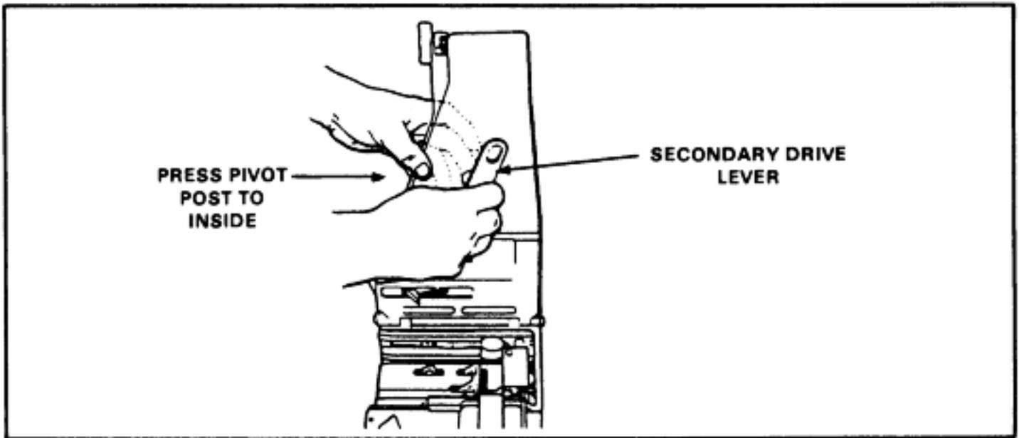
Figure 2-6. Secondary drive lever removal.
