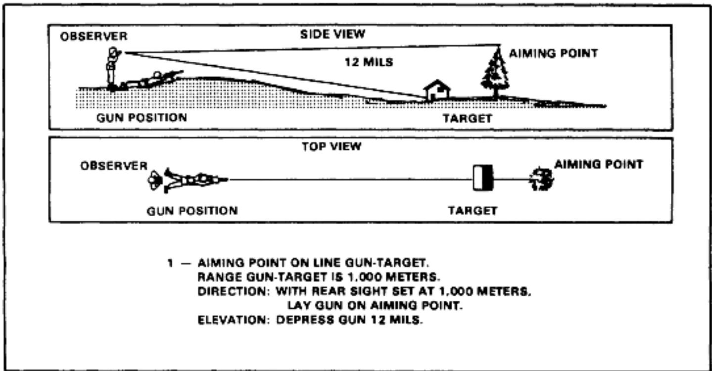
Figure 6-26. Aiming-point-method for elevation.
