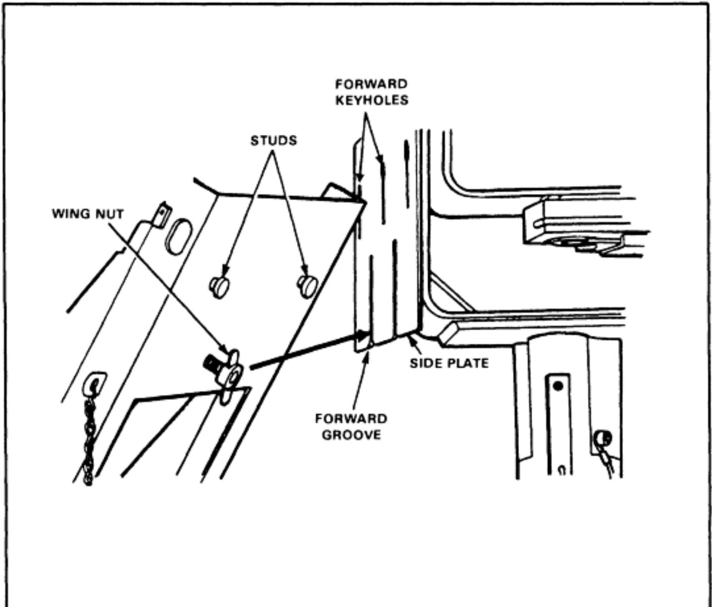
Figure 3-25. Attachment of bracket mounting assembly.
