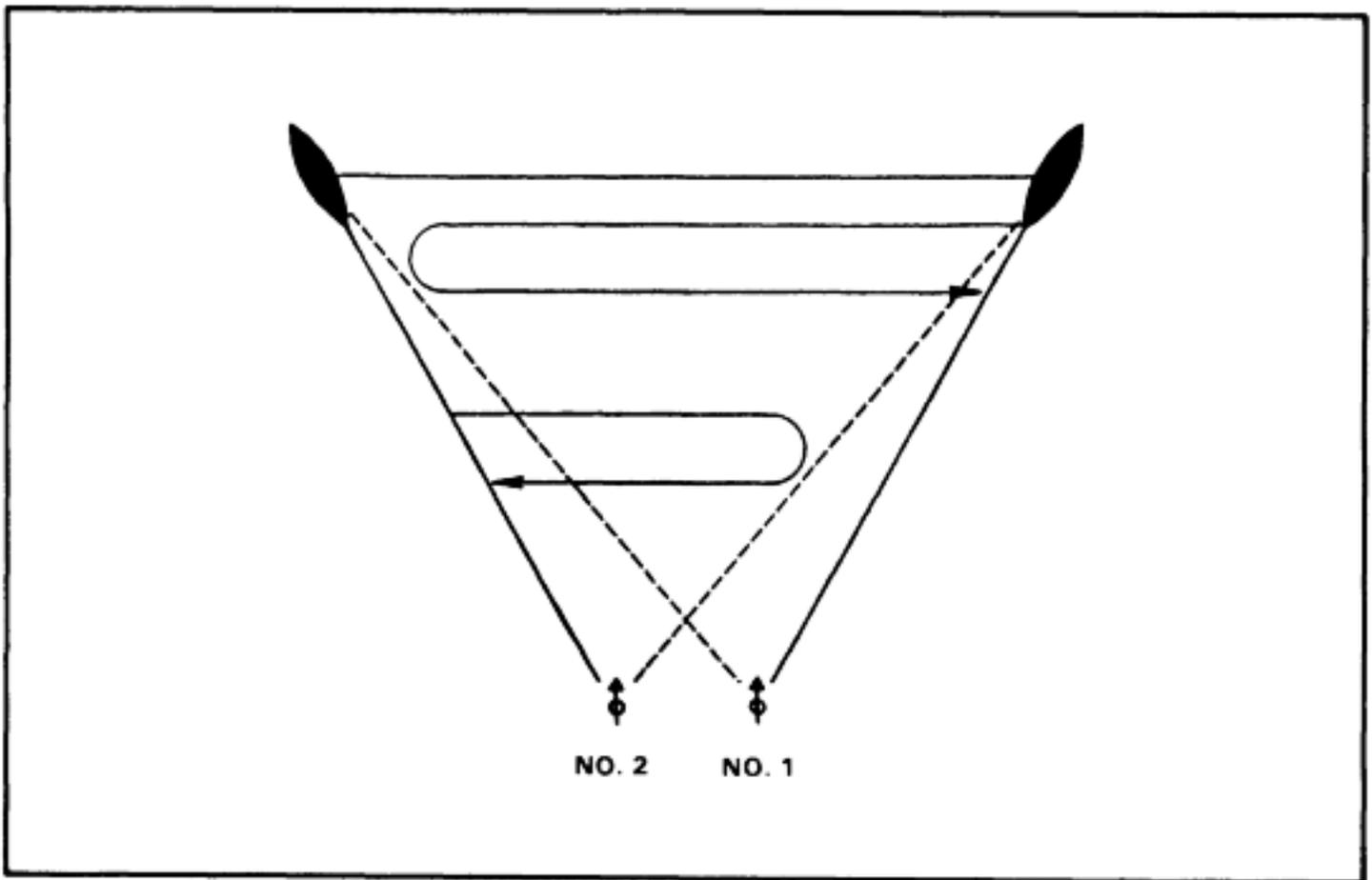
Figure 6-11. Traversing method, pair of MK 19s, target 100 mils or less in width, both flanks visible.
