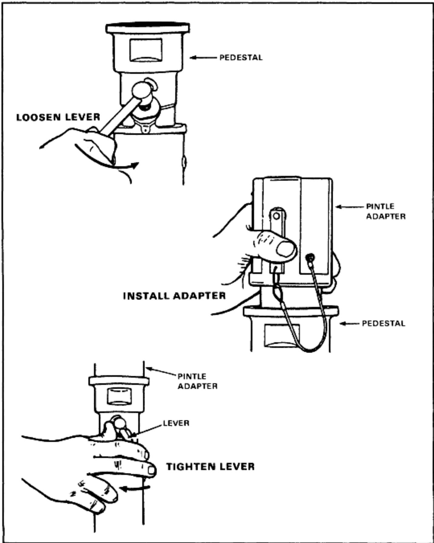
Figure 3-20. Pintle adapter installation.
