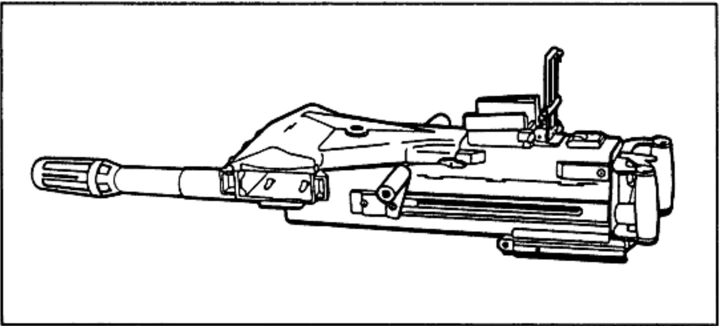
Figure 1-1. 40-mm grenade machine gun, MOD 3, MK 19.
