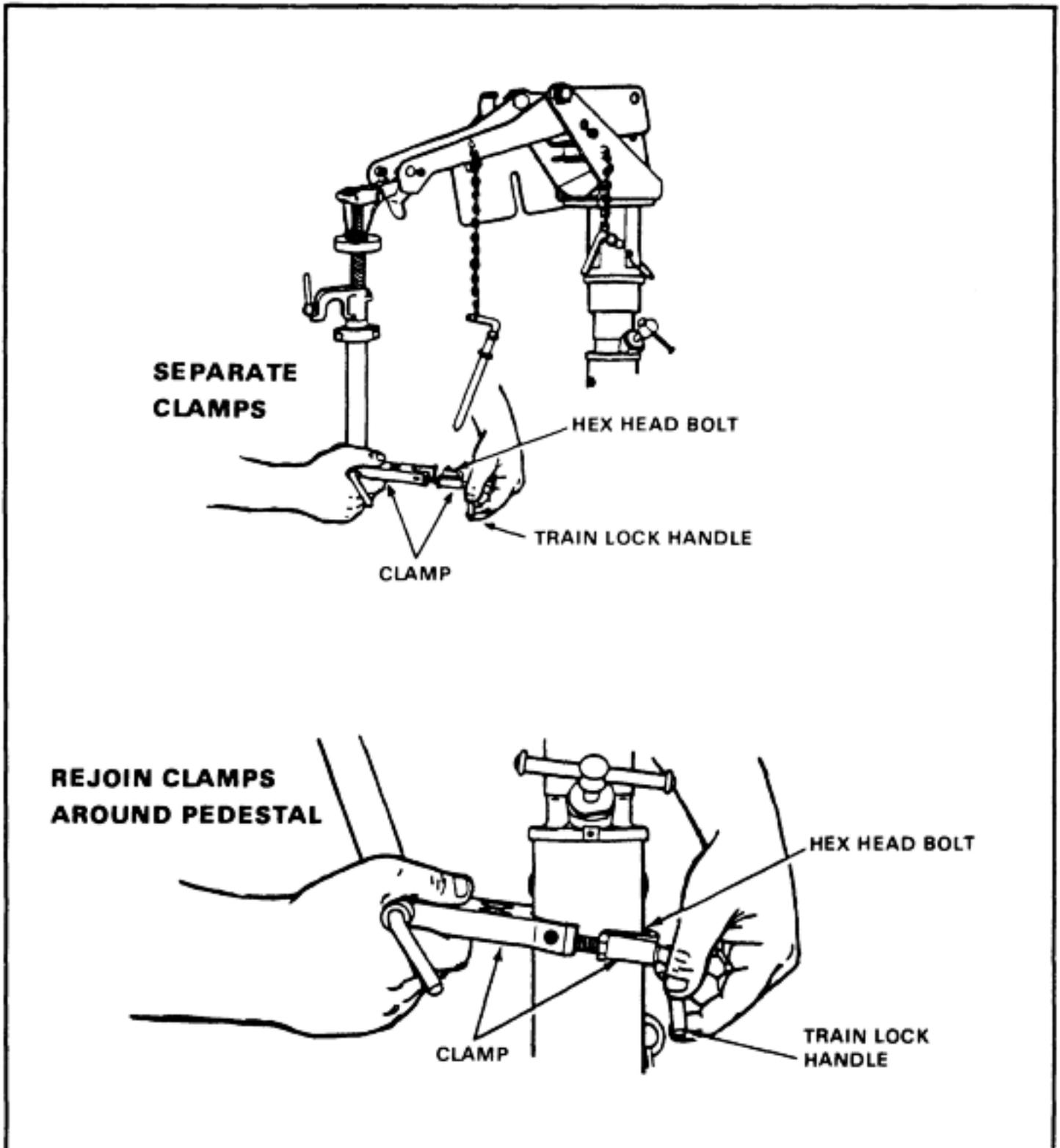
Figure 3-23. Train and elevating assembly installation, lower part.
