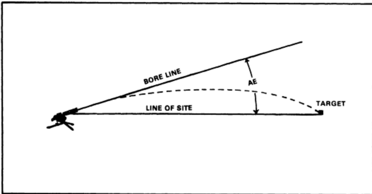
Figure 6-24. Angle of elevation.
