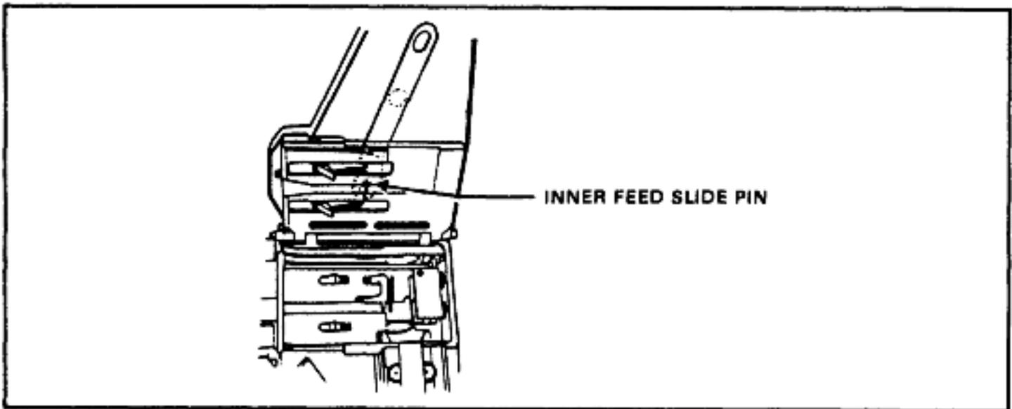
Figure 2-20. Replacement of secondary drive lever.
