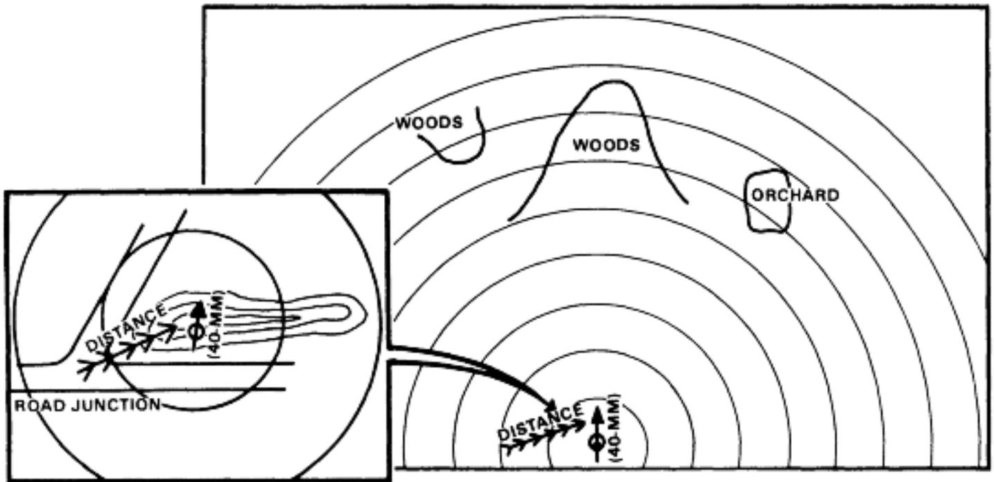
Figure 5-16. Distance and azimuth to terrain feature.
