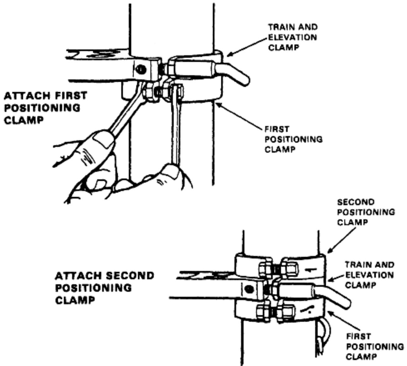
Figure 3-24. Attachment of positioning clamps.
