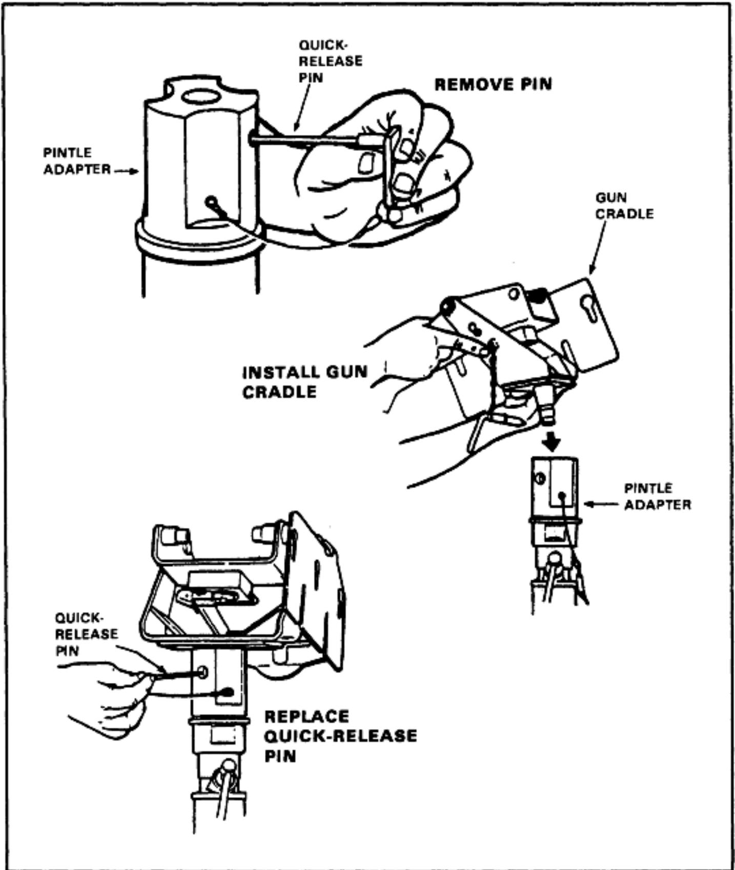
Figure 3-21. Gun cradle installation.
