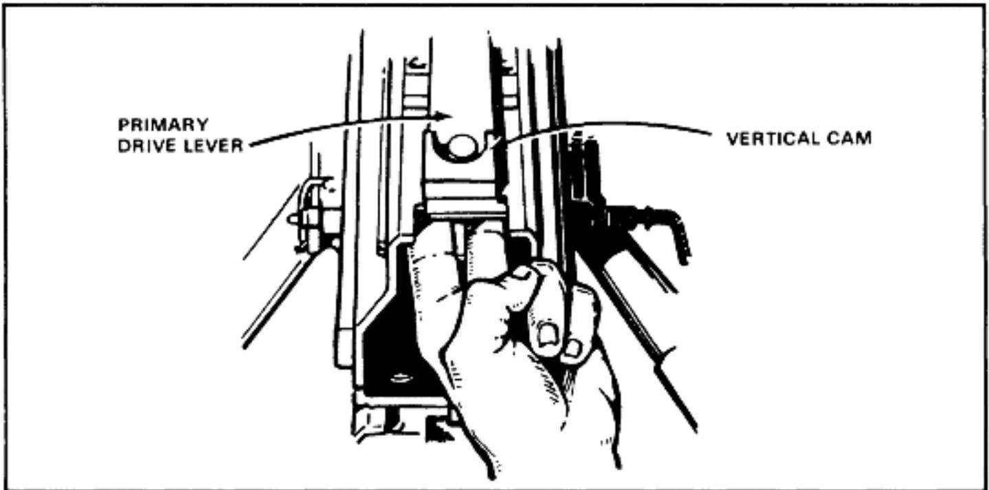
Figure 2-12. Primary drive lever and vertical cam.
