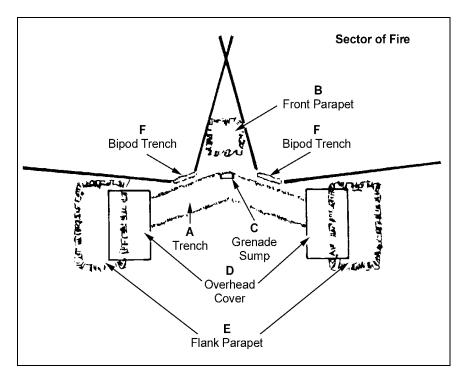
Figure 8-6. Construction of a two-man fighting position.
