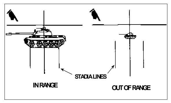
Figure 8-12. Range determination for flank target.
