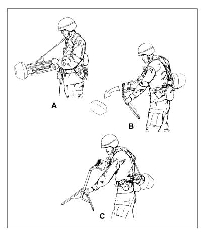
Figure 2-2. Releasing the bipod.
