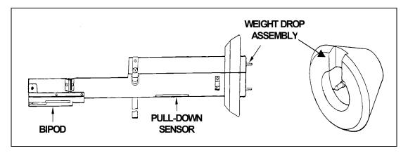
Figure B-13. Launcher and weight assembly.
