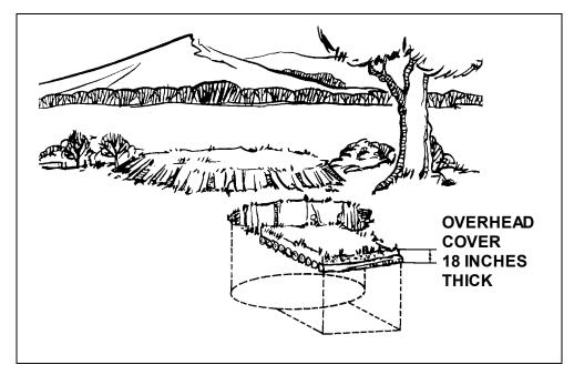
Figure 8-5. Construction of overhead cover.
