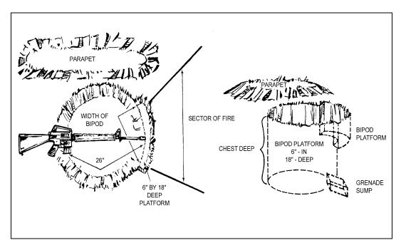
Figure 8-4. Construction of a one-person fighting position.
