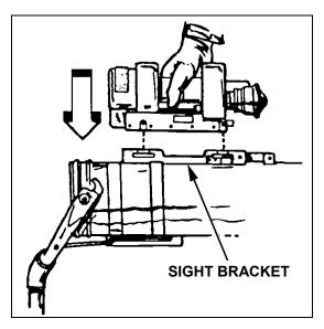
Figure 2-4. Aligning the daysight guide pins.
