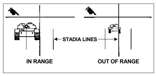
Figure 8-15. Range determination for frontal or rear target.
