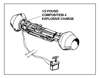
Figure H-1. Explosive charge on a round.
