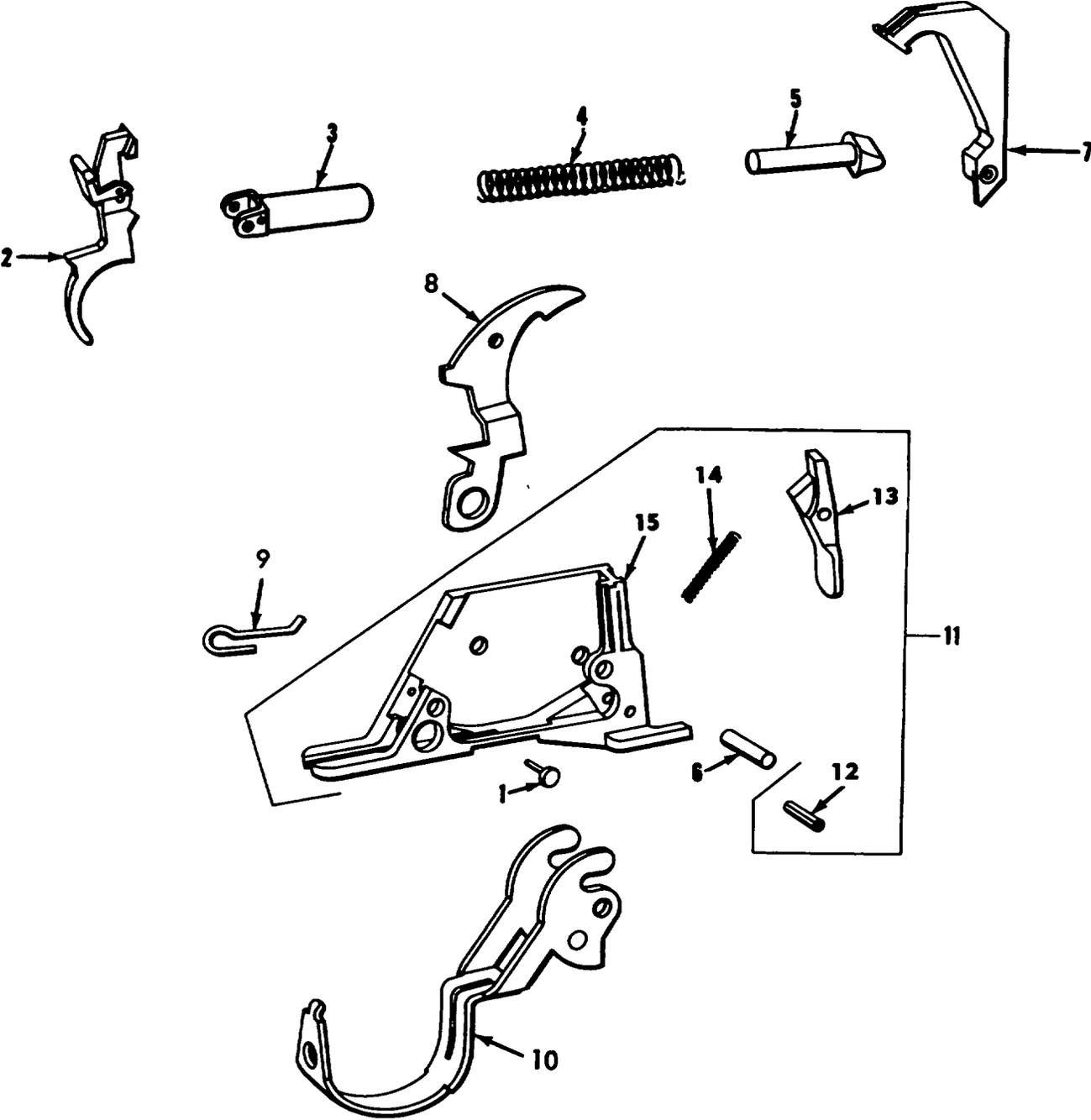
Figure 3. Firing mechanism-exploded view.
